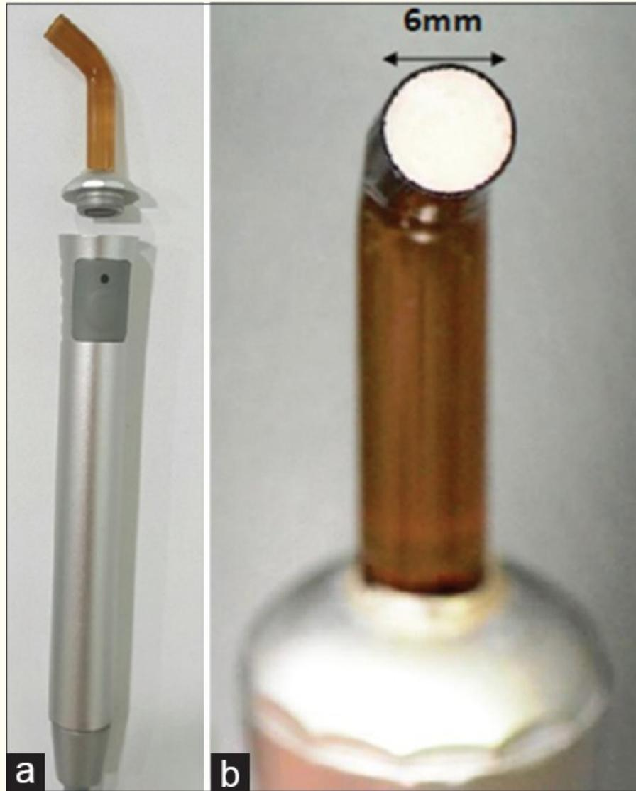
A photograph demonstrating a: the Pico T applicator unthreaded from the handpiece. b: The spot size of the Pico T applicator is 6 mm in diameter with a surface beam area of  $0.28 \text{ cm}^2$
