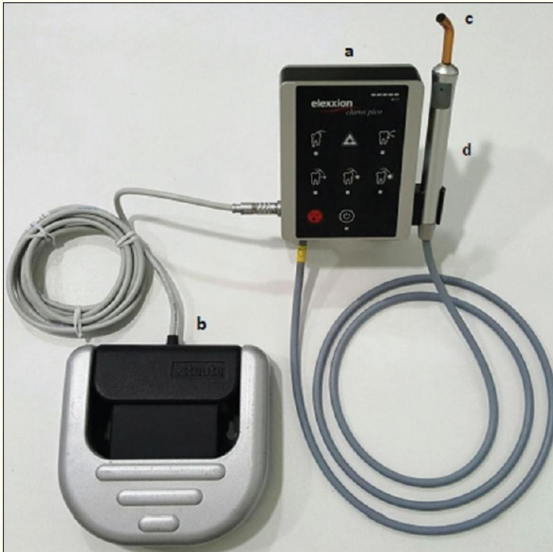
A photograph illustrating elexxion claros Pico laser device used. a: The display elements on the stand, b: The foot pedal for activation control, and c: The Pico T applicator fully threaded into the d: handpiece
